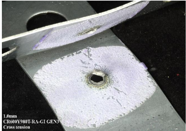
Button pull with cohesive separation
