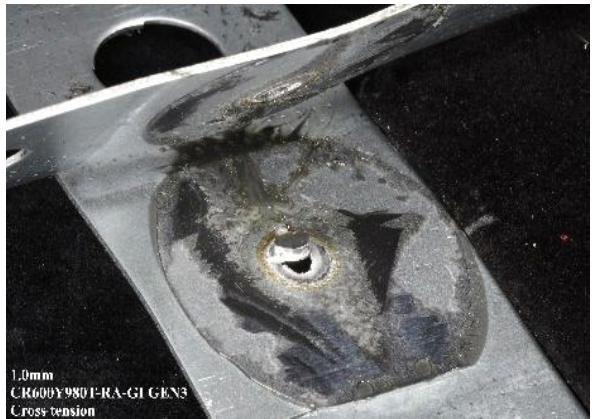
Button pull with adhesive separation
