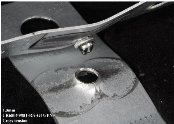
Rivet pull-out with adhesive fracture
