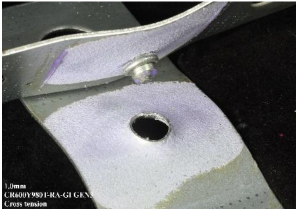
Rivet pull-out with cohesive fracture
