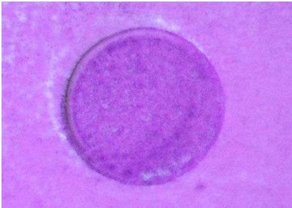
FLPI indications were not attributed to LME cracking.
