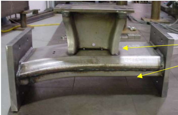
Frame sample with welded endplates
