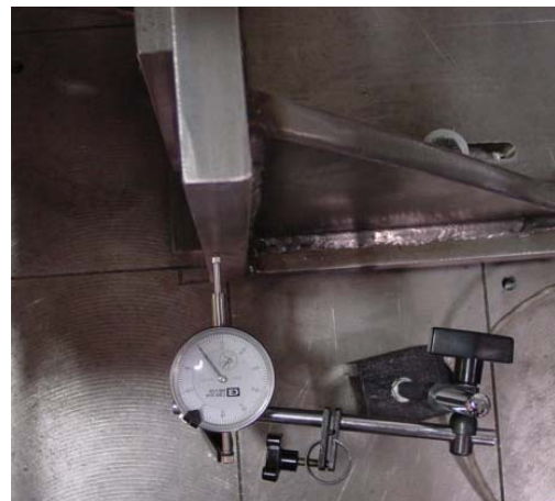
Dial indicator monitoring endplate movement
