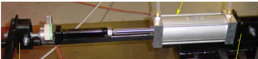
7" Stroke pneumatic cylinder with load cell and heim joint connections
