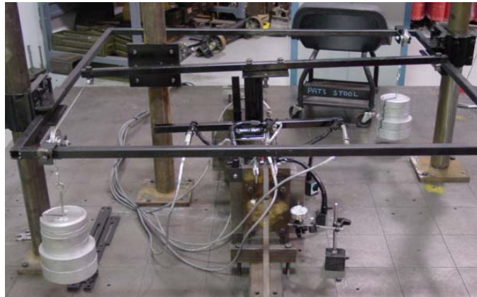
Torsion test setup including LVDT placement
