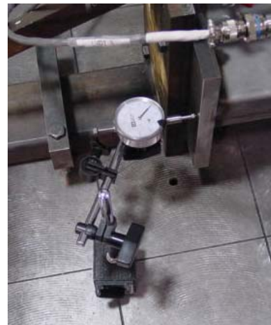
Dial indicator monitoring endplate movement
