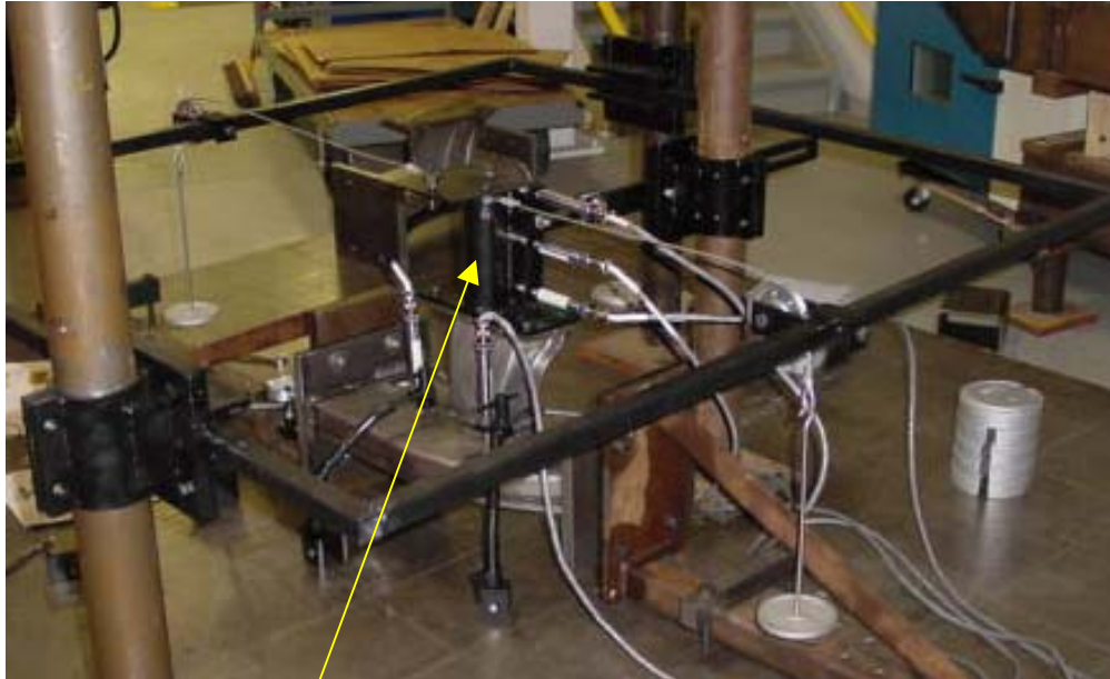
X direction test setup including LVDT positioning
